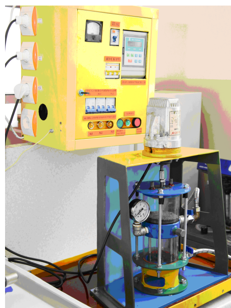
Fig. 3. The photograph of the working model of a vibro-cavitationator for homogenisation of blue-green algae biomass with a control panel for the power supply network
