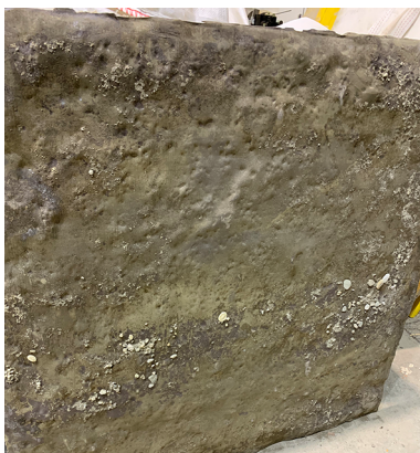
Fig. 3. The bottom of the CC layer after the test. No puncture happened, and the lower PVC layer was not torn
