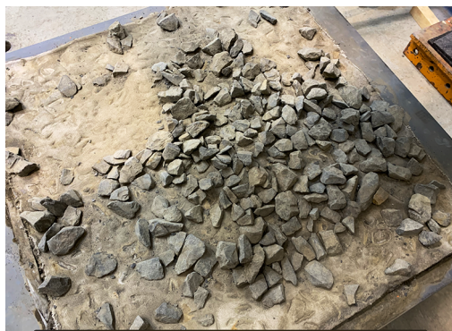
Fig. 8. The amount of the wedged, unmovable ballast particles after the test
