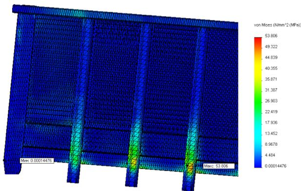
Fig. 5. A fragment (side wall) of the strength calculation results. Existing design scheme
