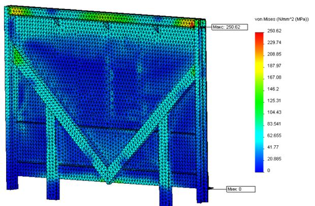
Fig. 4. A fragment (end wall) of the strength calculation results. Prospective design scheme
