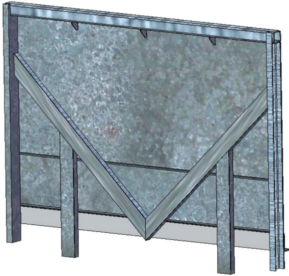
Fig. 2. End wall of freight wagon model 12-4745. Prospective design scheme
