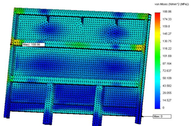
Fig. 3. A fragment (end wall) of the strength calculation results. Existing design scheme
