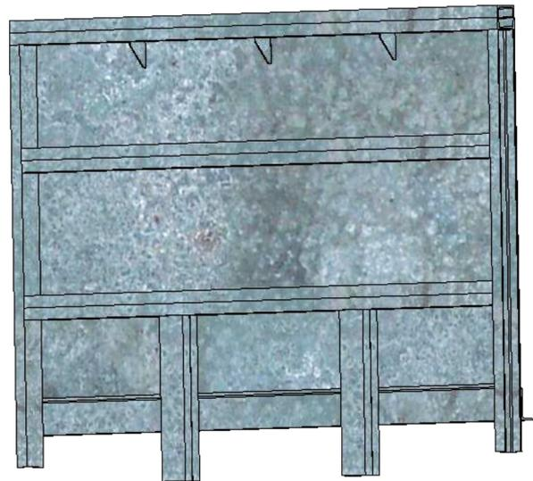
Fig. 1. End wall of freight wagon model 12-4745. Existing design scheme
