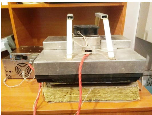
Fig. 2. Installation for moistening the material
