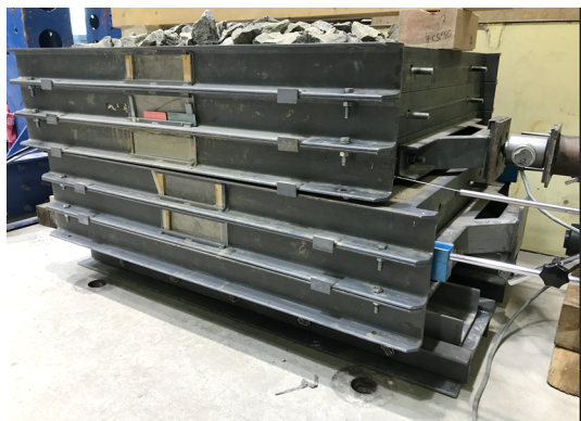
Fig. 4. The multi-level shear box during the shear test
