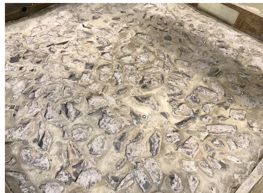
Fig. 5. The surface of the CC after the shear test
