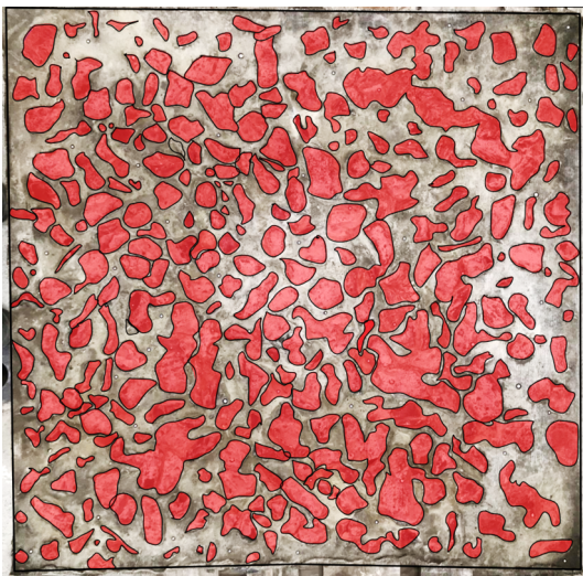
Fig. 7. Evaluation of the contact surface on a 1x1 m large CC sample
