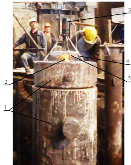
Fig. 9. Modification of the axial zone of a cast-iron rolled roll weighing 1115 kg with aluminum weighing 0.488 kg using a device with an electric motor:
