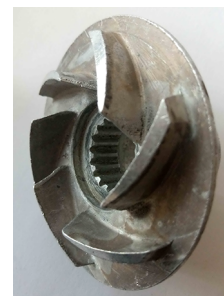
Fig. 11. Centrifugal pump impeller with a tapered inlet edge
