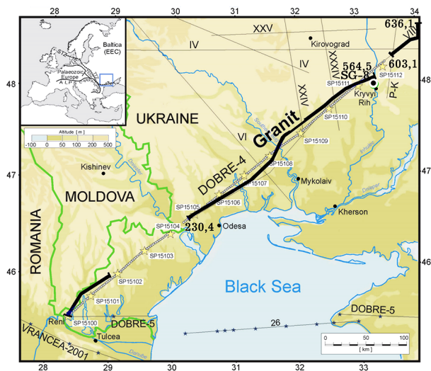
Fig. 1. Location of seismic geotraverses [6]: DOBRE-4, “Granit” and other DSS profiles; Kryvyi Rih superdeep well SG-8 [10] on the territory of Ukraine. Conventional annotations. Stars in yellow represent shot points; gray dots show recording stations of the DSS experiment; blue stars - survey points of the VRANCA-2001, DOBRE-5 experiments and recording devices along profile 26 (offshore part of DOBRE-5); black lines with Roman numbers – old DSS geotraverses; R-K, Putyvl- Kryvyi Rih profile; green lines are state borders. The inner map shows the location of the study area in Europe
