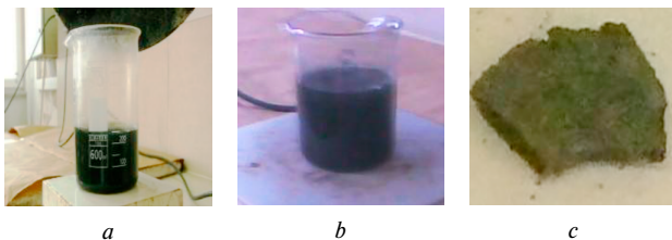
Fig. 1. Wastewater residues of refining processes: a – aqueous residues of PM; b – aqueous residues of PGM; c – filtrate after filtration process
