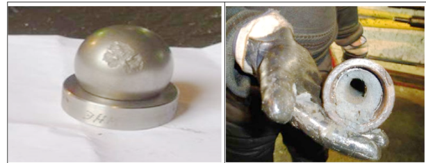
Fig. 2. Wear of a valve pair due to the ingress of mechanical impurities into the pump
