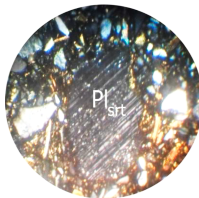
Fig. 4. Listvenite-beresite through rhyolite with relict porphyry structure of quartz-plagioclase phenocrysts. Bilozerska GSS. 90x zoom. Cross-polarized light
