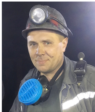
Fig. 1. Attachment of a personal SV 104 noise dosimeter to the employees' special clothes
