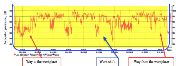
Fig. 2. Example of the processing of equivalent sound level measurements in Svantek Supervisor
