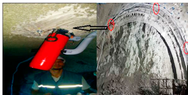
Fig. 4. Extensometer measurement system
