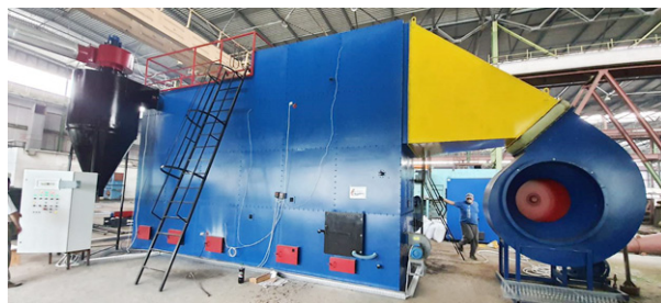
Fig. 1. Exploratory prototype of a 2500 kW heat generator-utilizer with the principle of vortex combustion of uncertified fuel
