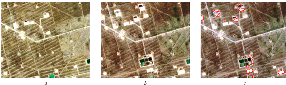
Fig. 9. An example of non-recognition of changes by two visible and infrared images from Sentinel-2A: a – 16.04.2017; b – 21.04.2018; c – recognition results
