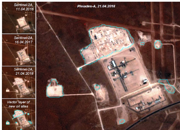
Fig. 6. Border accuracy assessment of new oil production sites in a given observation area from April 2016 to April 2018 according to visible and infrared images from Sentinel-2A
