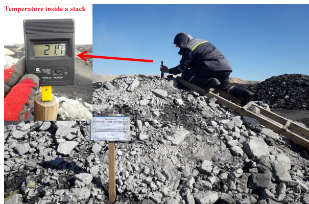
Fig. 9. Temperature measurement of a stack of polymer coated – “Techflex-M”
