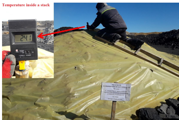
Fig. 8. Temperature measurement of a stack coated with a three-layer film
