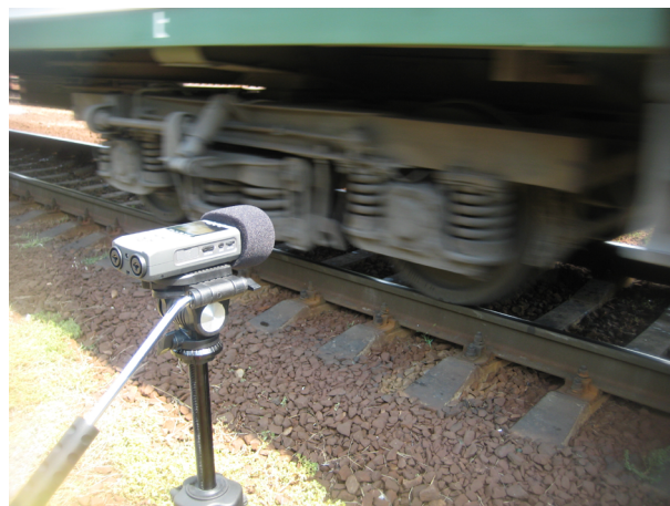
Fig. 1. Arrangement of the sound recorder relative to the train
