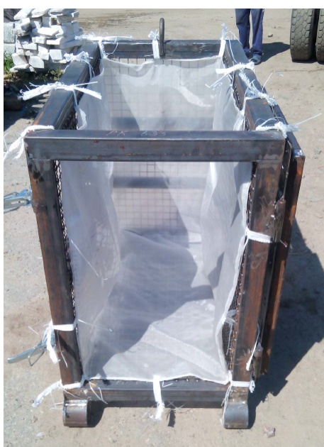
Fig. 4. Model of the mobile slurry container with a set up filter fabric bag
